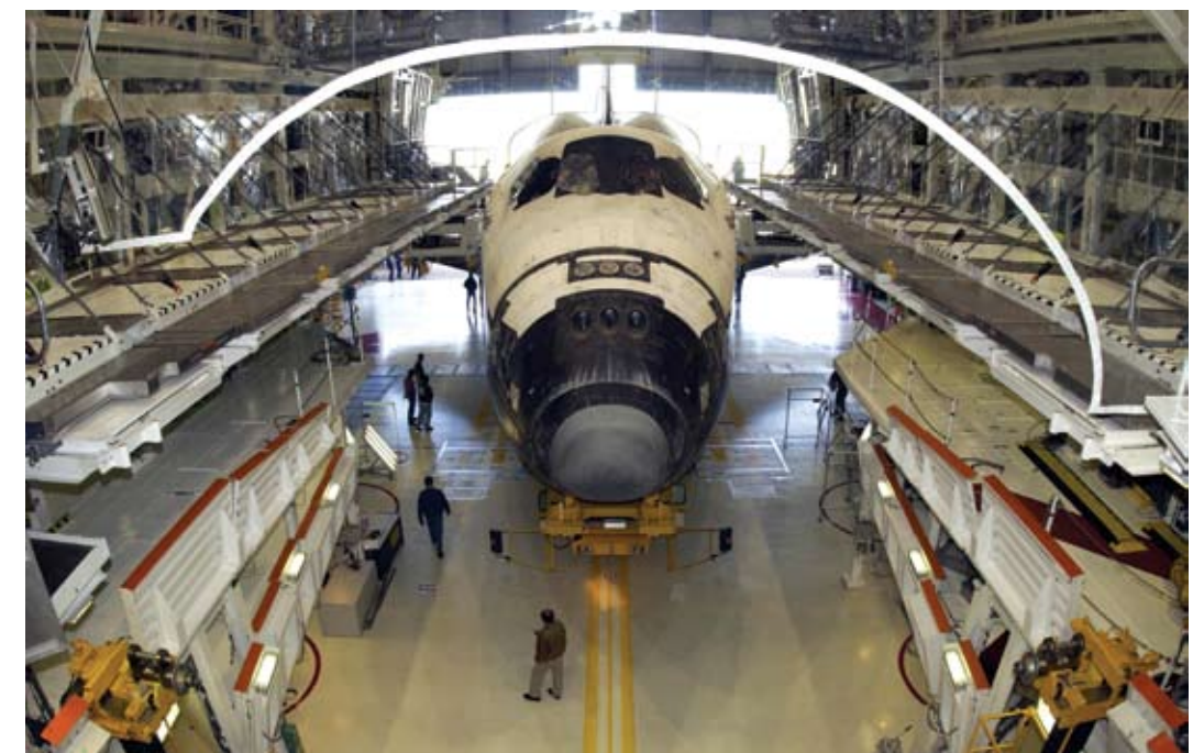
Orbiter Atlantis begins backing out of the Orbiter Processing Facility for rolover to the Vehicle Assembly Building, where it will be mated with the external tank and solid rocket boosters for launch.
