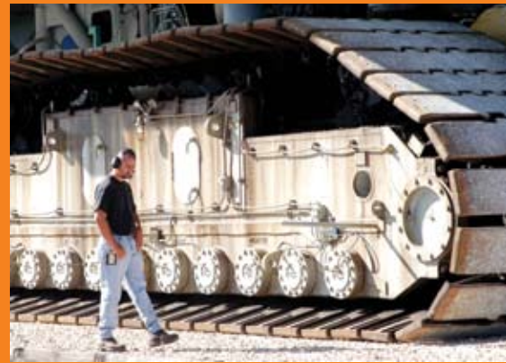
This Spaceport worker is dwarfed by the massive track of a crawler-transporter, which is used to carry a mobile launcher platform and space shuttle from the Vehicle Assembly Building to the launch pad. Space shuttle launch operations require experience and skills found nowhere else in the world.
