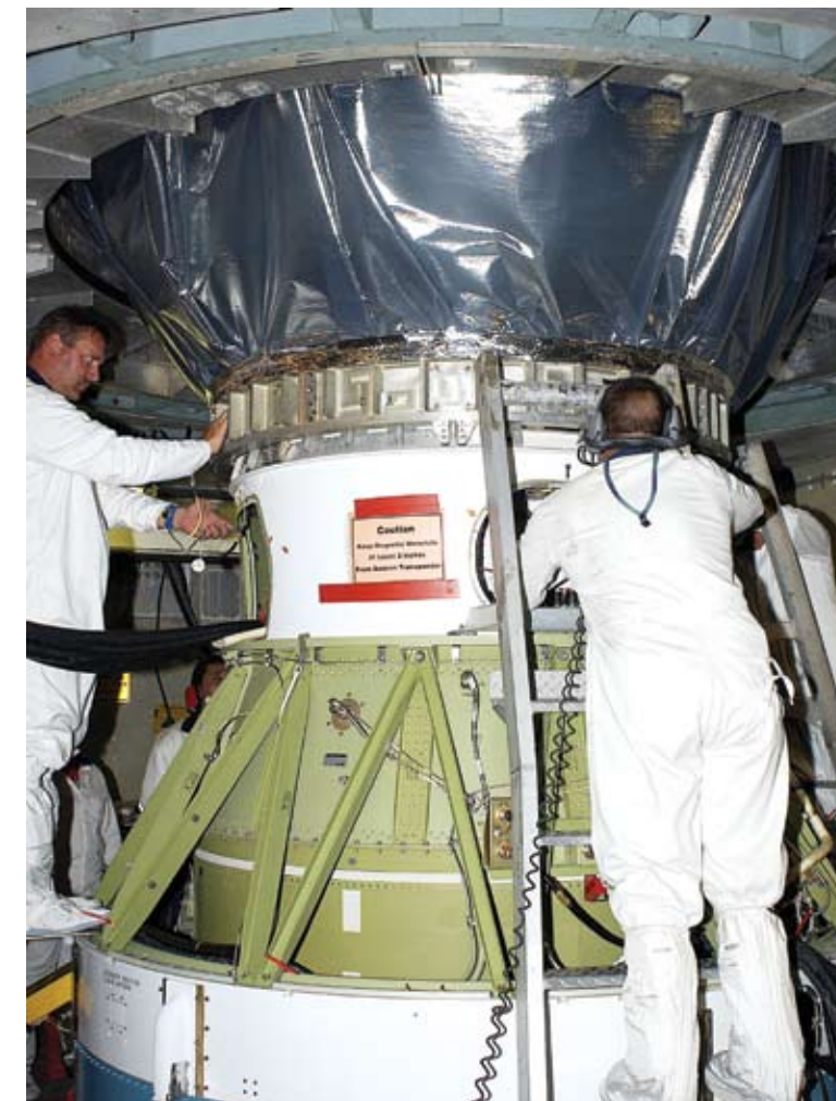
Workers on Launch Pad 17-B, Cape Canaveral Air Force Station, complete mating of the Mars Exploration Rover 1 (MER-B) above, to the Boeing Delta rocket below. The second of twin rovers sent to Mars, it is equipped with a robotic arm, a drilling tool, three spectrometers, and four pairs of cameras that allow it to have a human-like, 3-D view of the terrain. The rovers landed safely on Mars in 2004 and lasted much longer than the three months originally planned for. They provided spectacular views and data that is still being analyzed.
