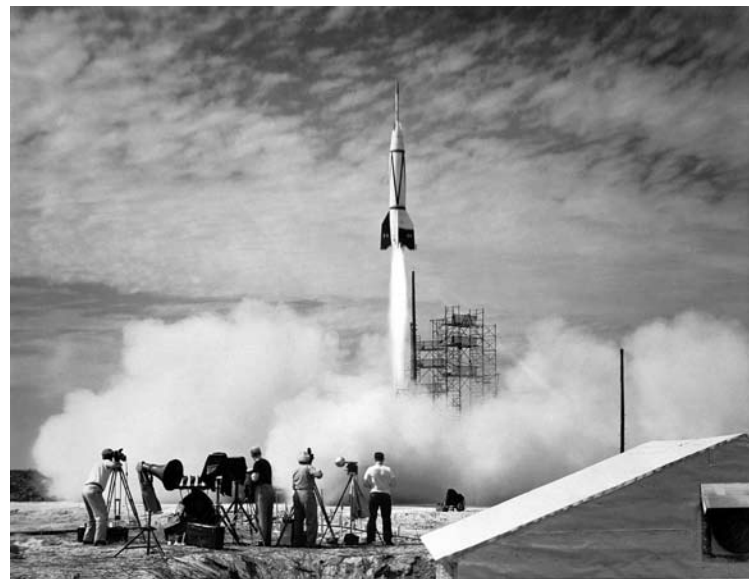
The first launch from Cape Canaveral – July 24, 1950. The modified German V-2 rocket attained an altitude of 10 miles. Note the primitive facilities: a tarpaper shack served as a blockhouse; the pad service structure was made from painters’ scaffolding.
