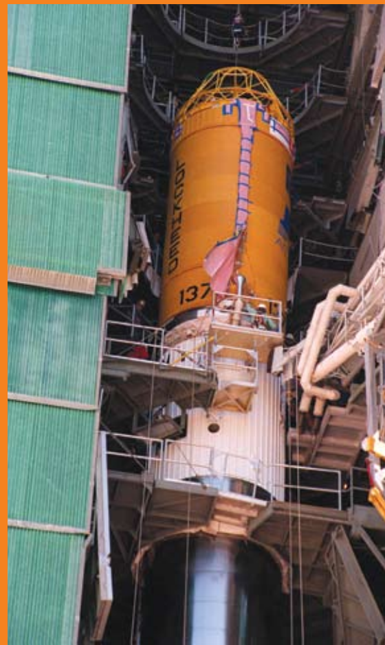
At Launch Pad 36-A, Cape Canaveral Air Force Station, a Centaur upper stage is mated to the lower stage Lockheed Martin Atlas IIA rocket. The rocket is scheduled to launch a NASA GOES satellite.
