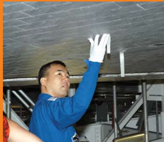
Readying a space shuttle orbiter for flight is an exacting job. Here Soichi Noguchi, with the Japan Aerospace Exploration Agency, JAXA, takes a close look at some of the tiles underneath Atlantis.
