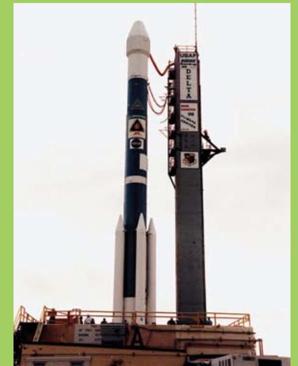
Protected by its gantry, a Delta rocket awaits launch under leaden skies at Complex 17. It later hurled a GOES weather satellite into a geostationary orbit. Three of the Delta’s five strap-on solid rocket boosters are visible in this photo.
