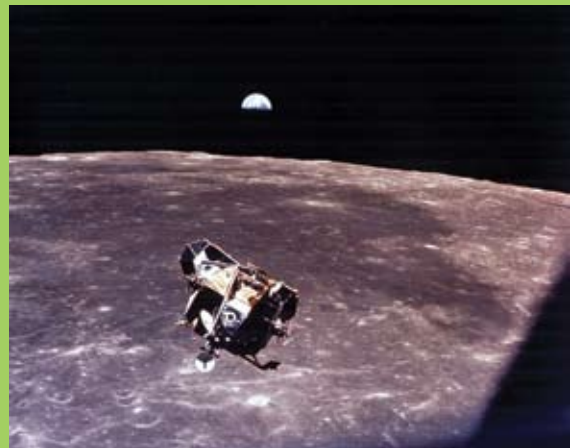
The ascent stage of the Apollo 11 Lunar Module floats over the eerie, crater-scarred landscape of the moon after Neil Armstrong and Edwin Aldrin Jr. successfully lifted off using the descent stage as a stable launch platform. This photo was taken through the orbiting Apollo spacecraft window by Michael Collins. After the rendezvous in orbit, the astronauts headed for Earth, seen here, half shadowed in darkness, above the bleak lunar horizon.
